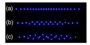
Figure 3.2: Different equilibrium structures: (a) linear string of ions, (b) two-dimensional zig-zag structure and (c) three-dimensional helix. Images like these are obtained by irradiating the ions with laser light of the appropriate frequency and detecting its fluorescence with a CCD camera.
