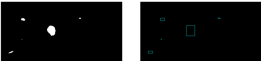
Fig. 4. left: hot spot image after classification in hot or cold pixels. right: visual representation of the results showing the location of the detected hot spot (the center of mass is not shown).
