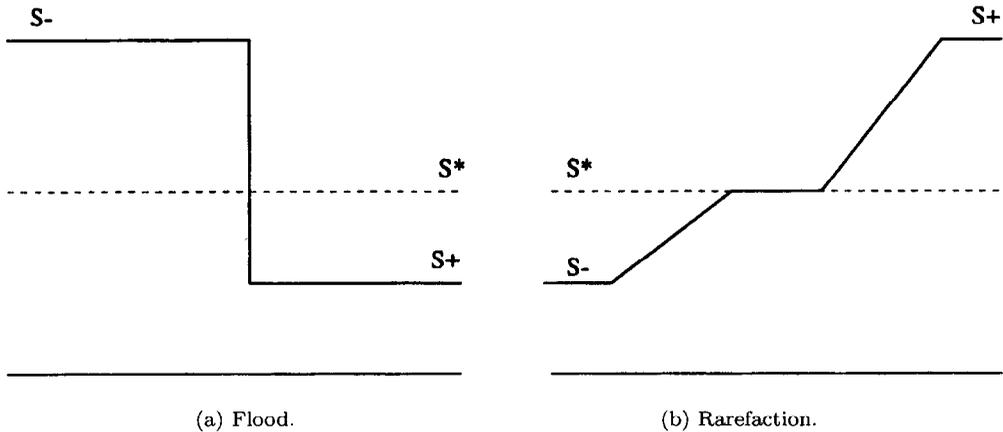
Figure 18. Solution to Riemann problems for a river trapped in a canyon.
