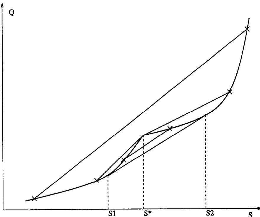
Figure 15. Convex and concave hulls of sections of the flux function for a river with flood plains.
