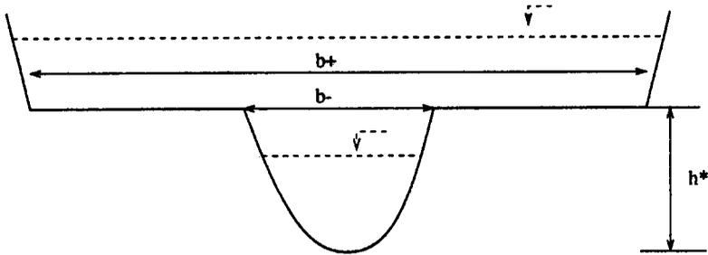
Figure 4. Schematic cross-section of a river with flood plains.
