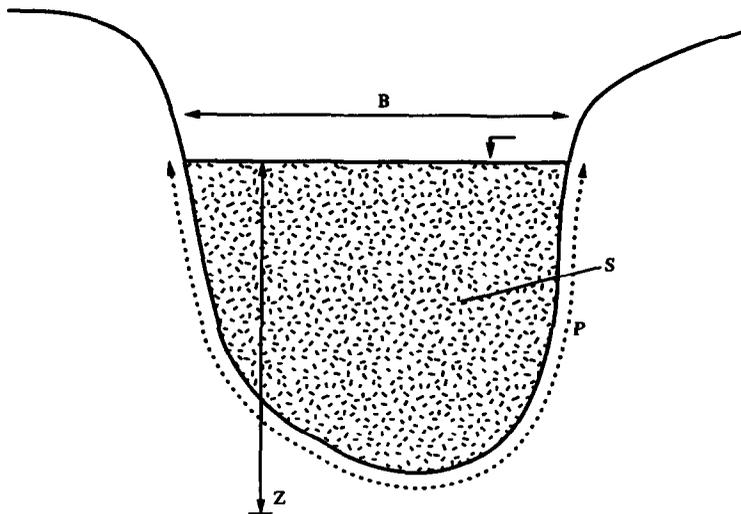
Figure 2. Schematic cross-section of a river. The variable  $S$  represents the wetted area,  $P$  the wetted perimeter, and  $B$  the surface width.
