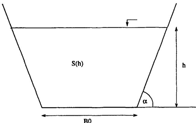
Figure 7. A trapezoidal cross-section.
