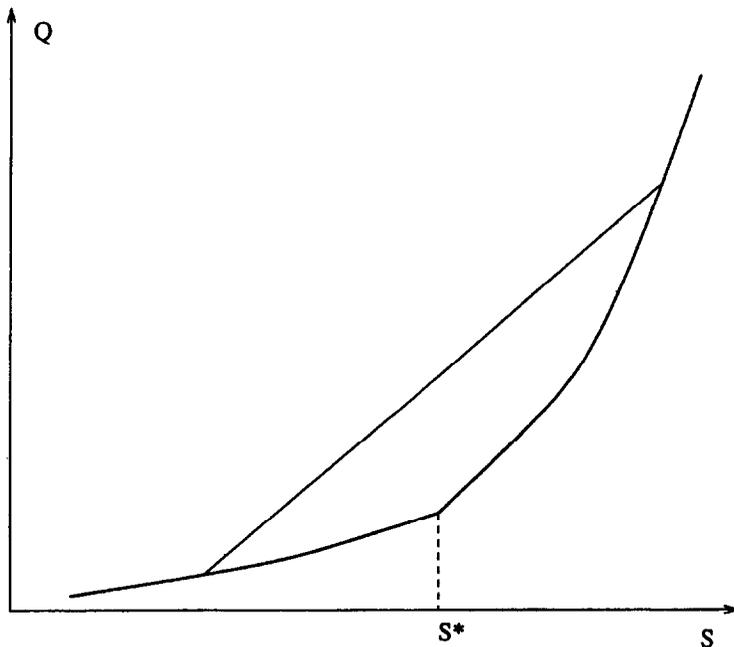
Figure 17. Convex hull of a section of the flux function for a river trapped in a canyon.
