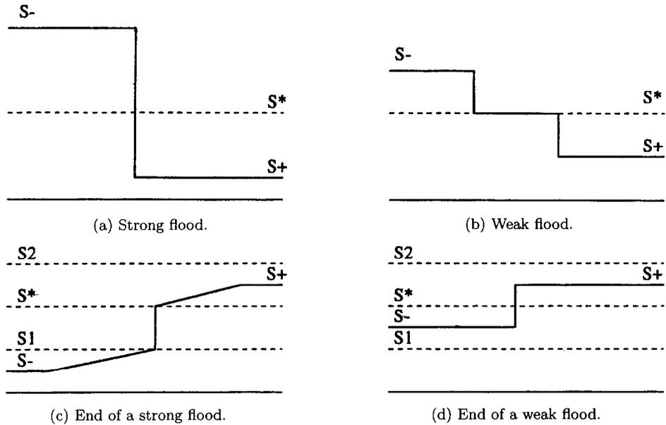
Figure 16. Solution to Riemann problems for a river with flood plains.
