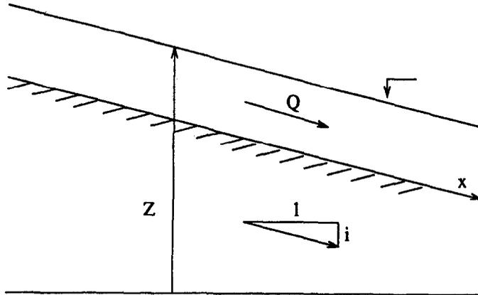
Figure 1. Schematic longitudinal section of a river. The variable  $x$  measures the length along the river,  $Z$  is the height of the water surface from a fixed horizontal reference plane,  $i$  is the surface slope, and  $Q$  the water flux per unit time.
