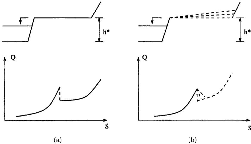
Figure 10. A Chézy model with uniform mean velocity for a river with flood plains, with and without bed slopes.
