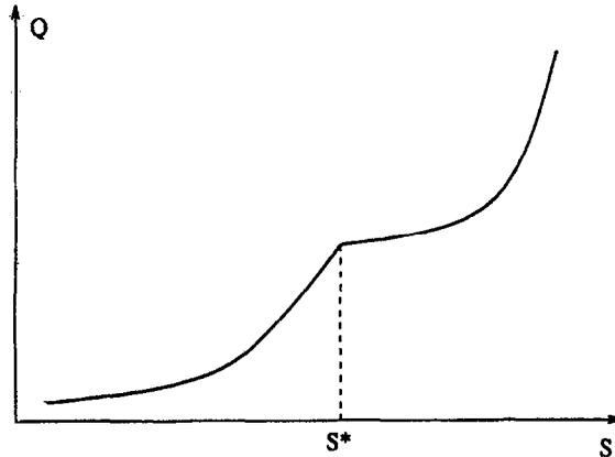
Figure 12. Flux function for a river with flood plains. The function is nonconvex, with a corner at the critical flood level  $S^*$ .
