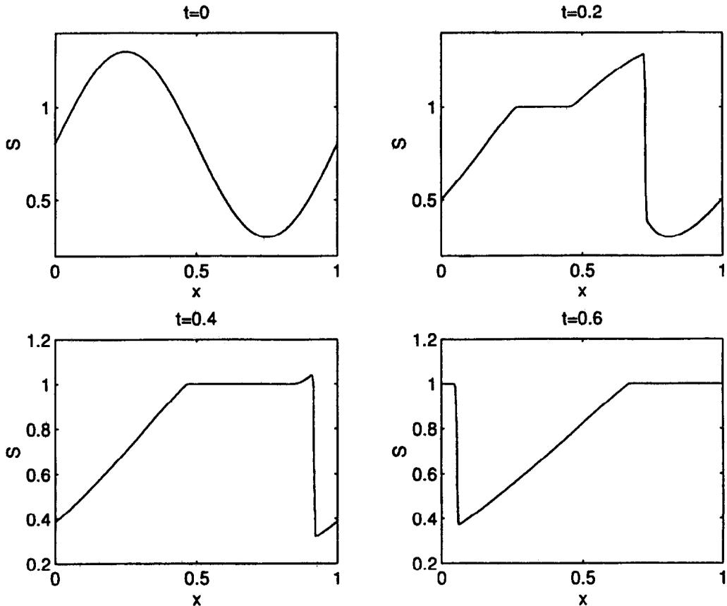
Figure 23. Numerical solution to the kinematic model for a river trapped in a canyon, on a periodic grid.
