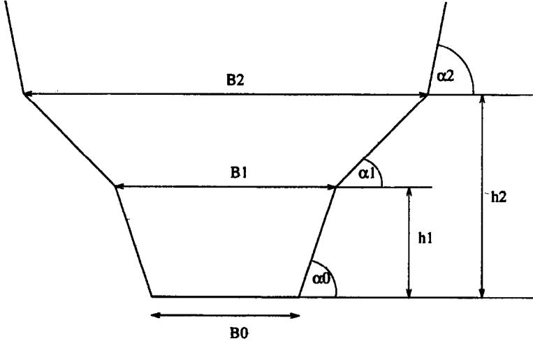
Figure 8. A piecewise trapezoidal cross-section.
