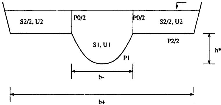
Figure 11. Improved model for a river with flood plains, with two mean velocities.
