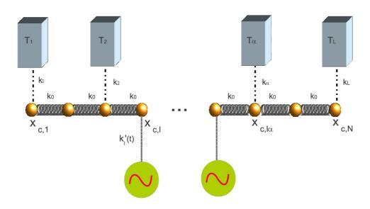
**Figure 1.** Sketch of the setup containing a central chain of acoustic phonons represented by a 1d lattice of atoms with equal masses connected by springs. This system is in contact to several reservoirs at different temperatures and affected by driving forces acting locally at the different positions of the central chain.
