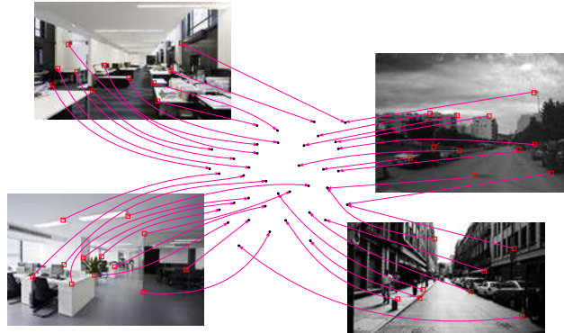
Figure 3.6: Extraction of descriptors from four sample images. The pink arrows indicate the association of each image feature with its corresponding descriptor. The set of points that are located in the middle of this figure reside in the descriptors space.
